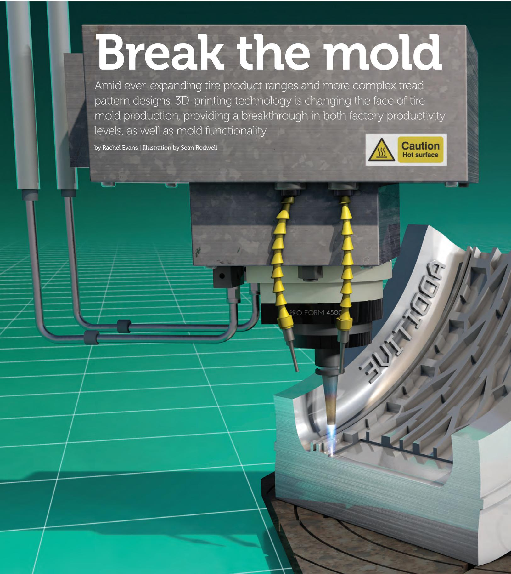
**I**n the production of tire molds, additive manufacturing is transforming the way segments are made, making revolutionary new tread pattern designs conceivable.
